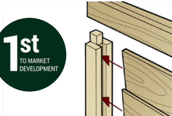
Rebated frame and Mortise and Tenon joint
