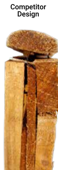
Capping rail 'popping off'
