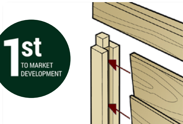
Rebated frame and Mortise and Tenon joint
