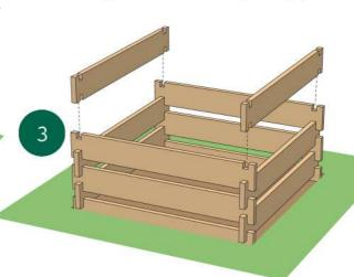
Finally, put the two remaining half-slats into position to complete the assembly.
