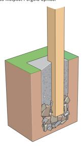
Whichever method is chosen, make regular checks with a spirit level, during the installation, to ensure that the posts remain vertical.
