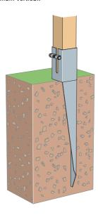
Site and install the posts using the chosen method of fixing. Use a spirit level during the installation to ensure that the posts are vertical.
