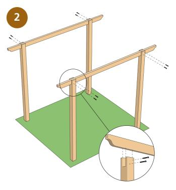
Drop a rafter into the Metclips and adjust to ensure that the overhang at each side is the same. Fix the rafter into position using screws or galvanised nails through the pre-drilled holes in the Metclips.
